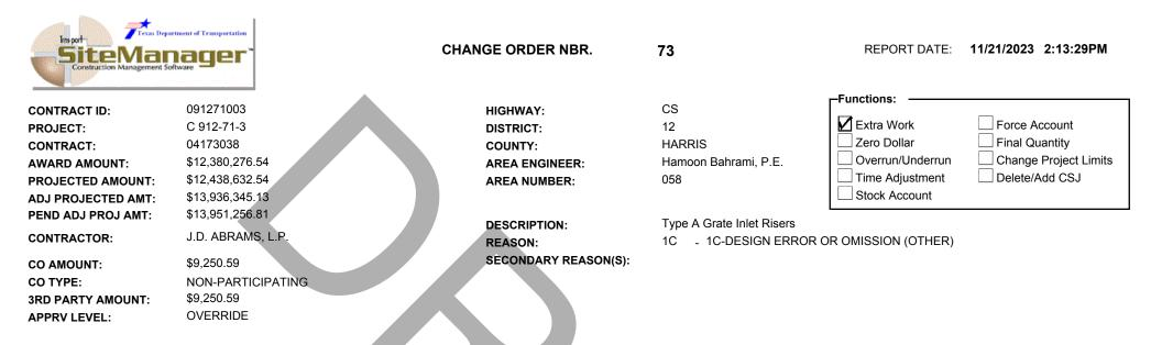
This change order will provide for adding one unique item of work to the contract to compensate the Contractor for the extra work performed to adjust the elevations of the Type A grate inlets installed inside the rain gardens.
